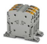
High-current terminal block, Blocked, Connection method: Power-Turn connection, Cross section: 10 mm<sup>2</sup> - 70 mm<sup>2</sup>, AWG: 8 - 2/0, Width: 60 mm, Height: 96 mm, Color: gray, Mounting type: NS 35/15
