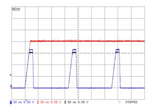
Since both Vo1 and Vo2 have the same delay and slew rate settings they will continue to turn off and on synchronously every 130ms as shown in Figure 34 until the condition causing the undervoltage is removed.
