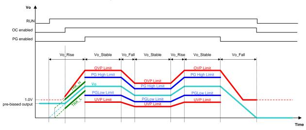
Figure 25. Protections Enable Conditions
