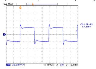
As the Load Regulation parameter is increased, step offsets in output voltage begin to appear, as shown in Figure 9.
