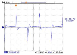
Figure 10. Transient Response with Optimal Voltage Positioning
