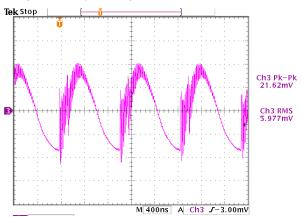
Figure 41. Output Voltage Noise, Full Load, 180° Interleave
