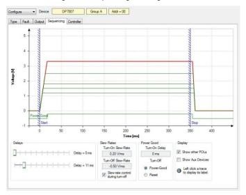
Figure 11. Sequencing/Tracking Window
