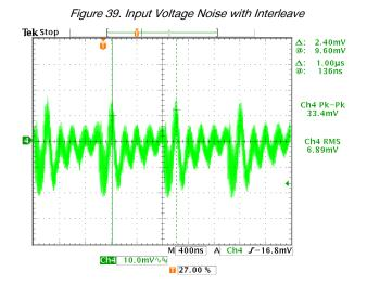
Figure 39 shows the input voltage noise of the three-output system with programmed interleave. Instead of all three dPOLs switching at the same time as in the previous example, the dPOLs V1, V2, and V3 switch at 67.5°, 180°, and 315°, respectively. Noise is spread evenly across the switching cycle resulting in more than 1.5 times reduction. To achieve similar noise reduction without the interleave will require the addition of an external LC filter.
