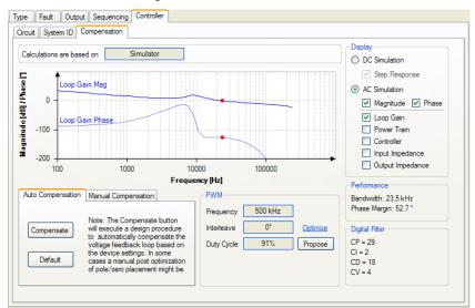
Figure 36. PWM Controller Window
