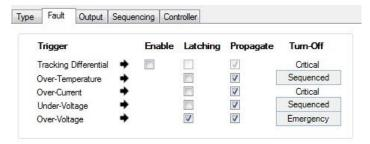
Figure 26. dPOL Fault Management Window
