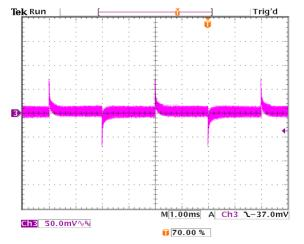
Figure 44. Transient Response with Regulation set to 3.72mV/A
