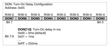
Figure 12. Turn-On Delay Register DON
