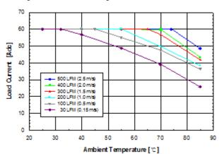
Figure 5. Thermal Derating Curves. Vin=12V, Vout=2.5V
