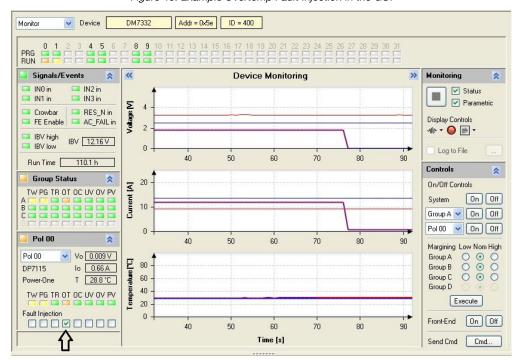
Figure 48. Example Overtemp Fault Injection in the GUI
