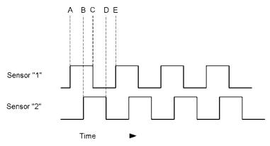
In the diagram, notice that after sensor 1 goes high (A), sensor 2 then goes high (B) as the encoder continues to rotate. Then, as the encoder continues to spin, sensor 1 goes low (C), and then sensor 2 follows (D). Because sensor 1 went high before sensor 2 (A-B), this indicates that the encoder disk is rotating in one direction (in the case of a robot, either forward or reverse). If sensor 2 went high before sensor 1, then the disk is rotating in the opposite direction.
