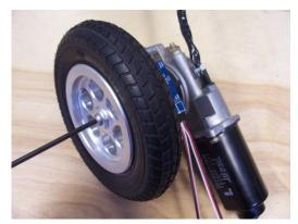
Step 12: Attach the Encoder PCB using two # 4-40 x 1/8" flat head Philips screws, as shown.
