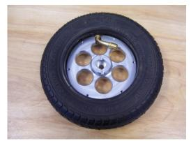
**Step 8:** Sandwich the two rims together, and secure with (6) #4-40 x ½" Flat Head Philips screws.
