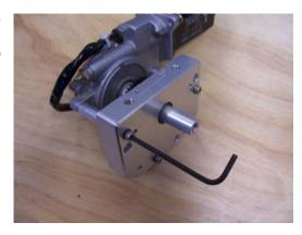
**Step 5:** Insert the drive pin into the hole in the axle. You may want to place the axle against a wooden block as you gently drive the pin half-way through the axle. The pin should be a very tight fit, and it should be centered in the axle as shown here. Tighten the (3) socket-cap screws.
