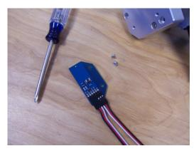
**Step 10:** Attach the Quadrature Encoder board to the Bearing Block as shown, using (2) 3/16 x 4-40 Flat Head Philips screws. Be sure that the Encoder Disc is centered within the Encoder sensor's slot.
