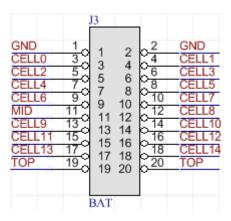
**Figure 3: Battery Connector**
