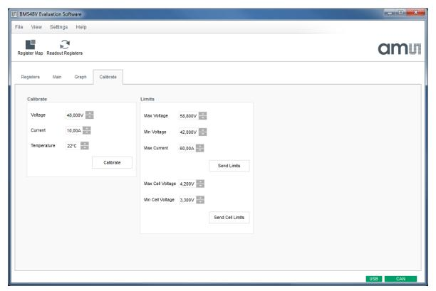
Figure 6: GUI Calibrate Tab
