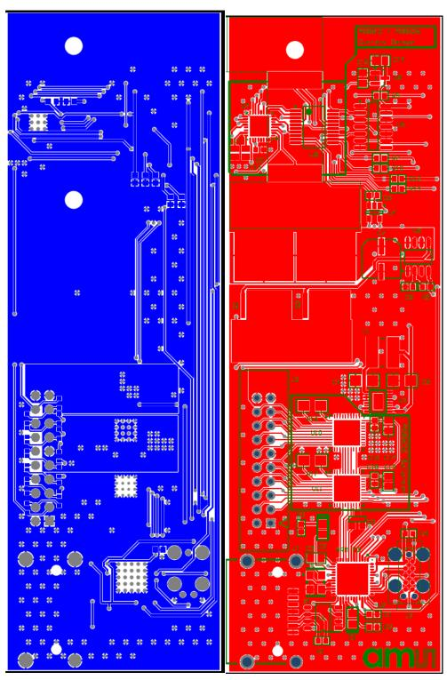
Figure 8: Top/Bottom PCB Side
