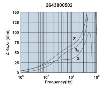
Impedance, reactance, and resistance vs. frequency.
