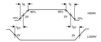
Figure 4. Output Drive Timing Diagram
