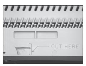
4.09 Lay at least 1 1/2 loops of fiber from the first buffer tube of the second cable on the tray with the fiber ends crossing the back "CUT HERE" mark.
