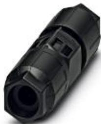
Conductor connectors, QUICKON connection, number of positions: 3+PE, 1 mm<sup>2</sup> ... 2.5 mm<sup>2</sup>, 690 V, 20 A, black, With two QUICKON nuts, cable diameter range: 6 mm ... 10 mm, QUICKON fast connection
