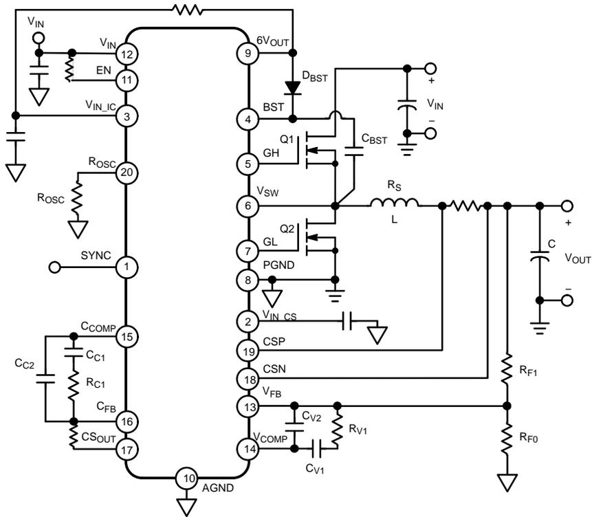
Figure 2. NCV8851B Application Diagram
