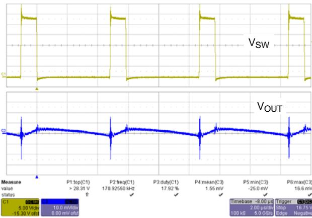
Figure 8. S<sub>WN</sub>, V<sub>OUT</sub> at 170 kHz, 28 V to 5 V Output
