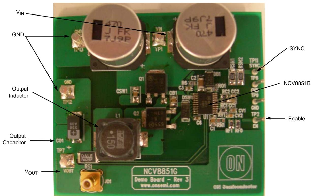
Figure 1. NCV8851B Evaluation Board
