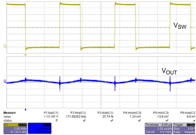
Figure 5. S<sub>WN</sub>, V<sub>OUT</sub> at 170 kHz, 13.2 V to 5 V Output
