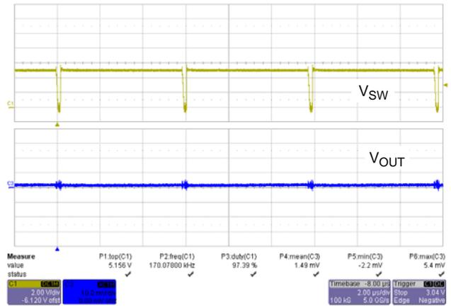
Figure 7. Maximum Duty Cycle at 170 kHz, 5 V Output
