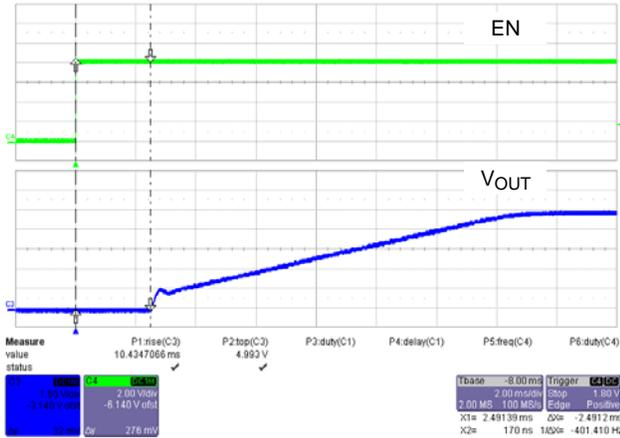
Figure 4. Startup at 170 kHz, 13.2 V to 5 V Output
