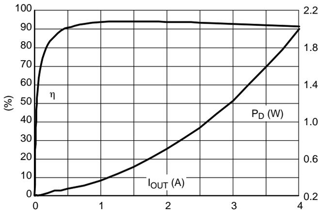
Figure 12. Efficiency at 170 kHz, 13.2 V to 5 V Output
