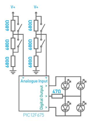
At the heart of the electronic circuit is a microcontroller. A microcontroller is, in effect, a small computer. The circuit uses a cleaver design to allow four switches and four LEDs to be connected to only five input / outputs.
