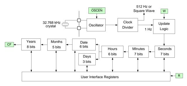
Figure 7. Real-time Clock Core Block Diagram
