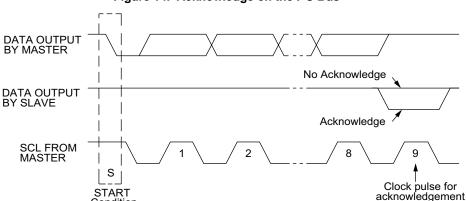
Figure 14. Acknowledge on the I<sup>2</sup>C Bus
