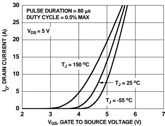
**Figure 5. Transfer Characteristics**
