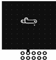
a.  $53\text{ }^\circ\text{C/W}$  when mounted on a  $1\text{ in}^2$  pad of 2 oz copper
