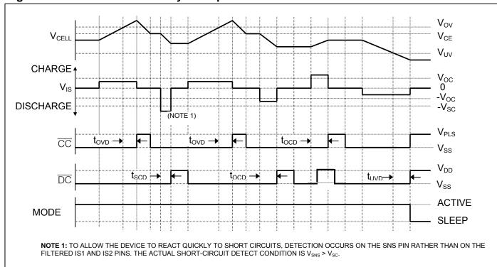
Figure 4. Li+ Protection Circuitry Example Waveforms
