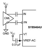
Figure 3d. CML Interface (AC-Coupled)
