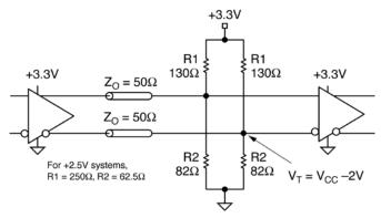
Figure 4a. Parallel Termination-Thevenin Equivalent
