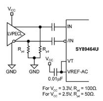
Figure 3b. LVPECL Interface (AC-Coupled)
