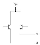
Figure 2b. Simplified Differential Output Stage
