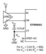
Figure 3a. LVPECL Interface (DC-Coupled)
