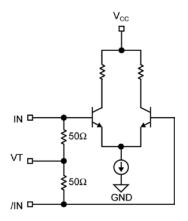
Figure 2a. Simplified Differential Input Stage
