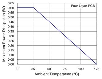
Figure 8. Derating Curves for the RT8241D Package
