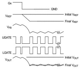
Figure 3. Output Voltage Down Transition
