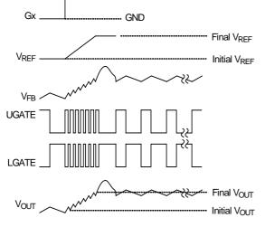
Figure 5. Output Voltage Up Transition with Overshooting
