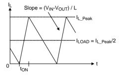
Figure 1. Boundary Condition of CCM/DCM
