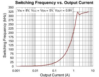
Switching Frequency vs. Output Current
