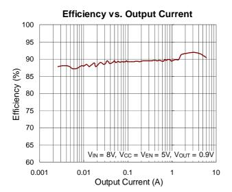
Efficiency vs. Output Current
