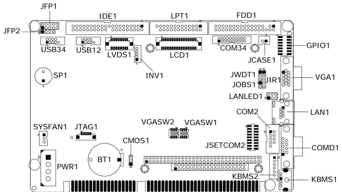
Figure 2.1 Jumper and Connector Locations (Component Side)
