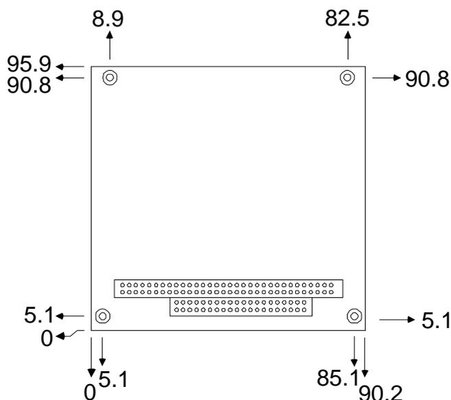
**Figure D.2 PC/104 Module Dimensions (mm) ( $\pm 0.1$ )**
