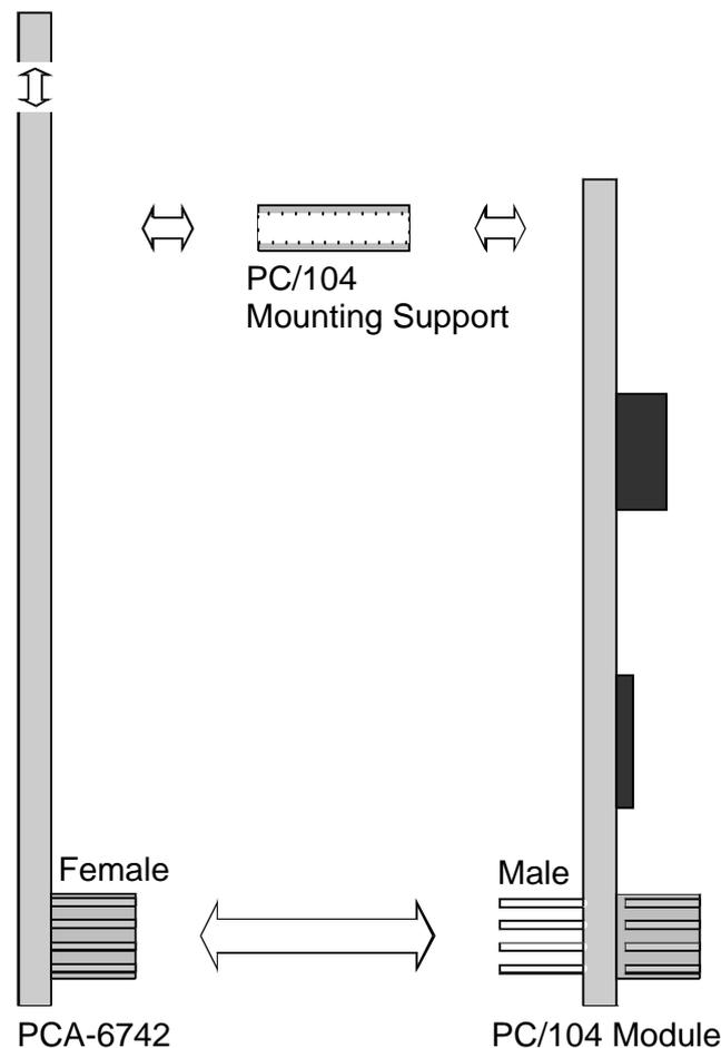
**Figure D.1 PC/104 Module Mounting Diagram**
