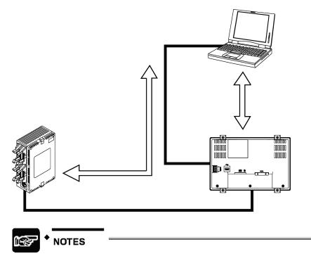
The system should be set up so that the Timeout period in the FP series software (A) is larger than the waiting time for communication retries of the GT COM port (B), meaning (A) > (B). If the system is set up so that A = B or A < B, the through function will not work properly.</li>
