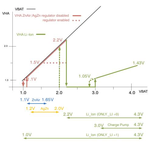
Figure 4. Hearing Aid Mode: Voltage Monitoring
