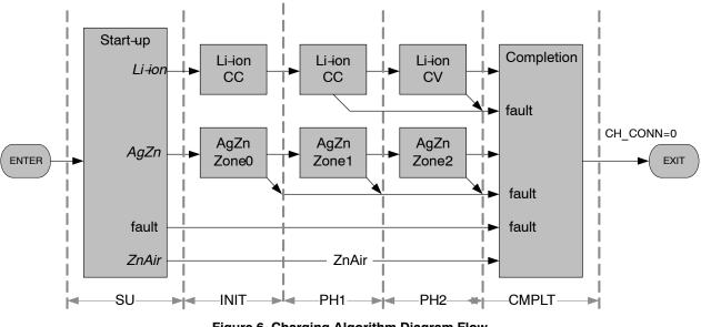
Figure 6. Charging Algorithm Diagram Flow
