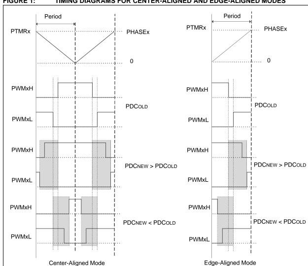
FIGURE 1: TIMING DIAGRAMS FOR CENTER-ALIGNED AND EDGE-ALIGNED MODES
