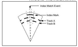
As a result of this, the value of POSxCNT may leave its expected range of 0 to maximum count (defined as the number of encoder pulses per revolution, minus 1), resulting in erroneous reporting of the rotor's position.
