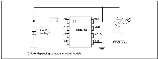
In addition to the IC, all that is required is a circuit for transmitting the information over the desired media (e.g., a UHF radio transmitter), a battery, and a button switch as shown in Figure 5-1. A single encoder can command a multifunction decoder to activate up to 15 specific functions/outputs. The user would select the desired function pressing one or more buttons on the transmitter.
