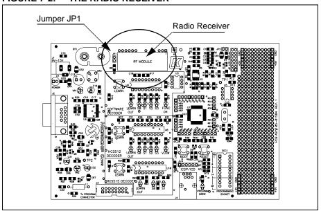
Jumper JP1 allows the radio receiver output to be disconnected from the decoders. This permits monitoring the receiver output on an oscilloscope or injecting an encoder's digital output directly into the decoder
