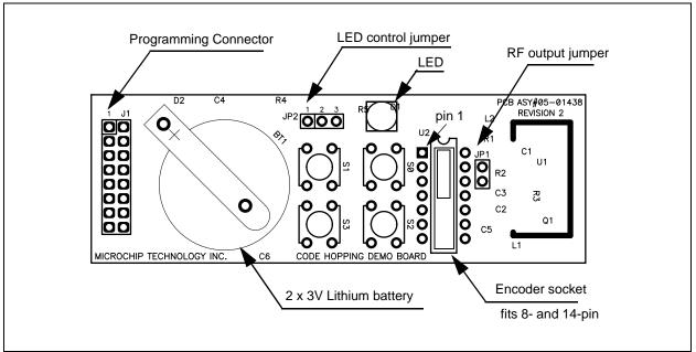
The **battery holder BT1** accepts one or two CR2016 3V lithium batteries, positive side up. While most encoder models will demonstrate reliable operation down to 2V, the demo RF oscillator circuit is only ensured to operate properly down to 4.5V.
