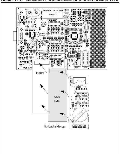
FIGURE 7-12: IN-CIRCUIT PROGRAMMING OF A DEMO TRANSMITTER
