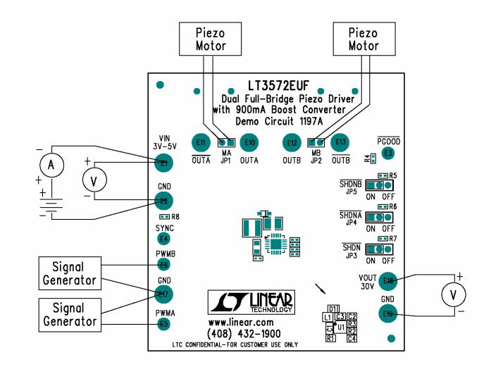
Figure 1. Proper Measurement Equipment Setup
