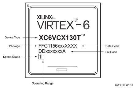
Figure 1: Example Device Top Mark
