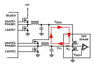
FIGURE 6. V<sub>TT</sub> CURRENT SINKING LOOP
