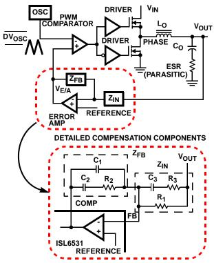
FIGURE 8. VOLTAGE-MODE BUCK CONVERTER COMPENSATION DESIGN
