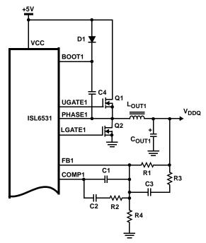
FIGURE 3. OUTPUT VOLTAGE SELECTION OF VDDQ
