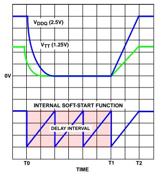
FIGURE 5. OVERCURRENT PROTECTION RESPONSE
