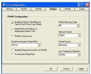
Figure 8: Fan Configuration
