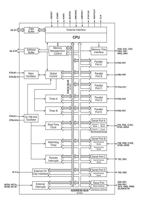
Figure 1-1. Block Diagram of the Rabbit Microprocessor
