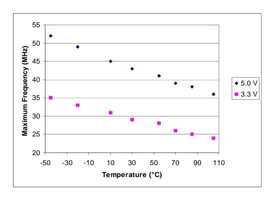
Figure 15-1. Rabbit 2000 Typical Maximum Operating Frequency versus Temperature at 5 V and 3.3 V
