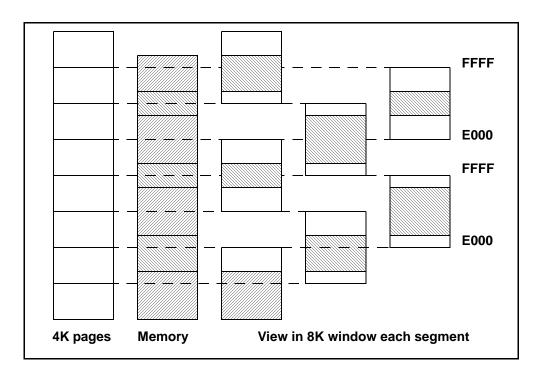
Figure 8-4. Compilation of Code Segments in Extended Memory
