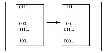
Figure 3-7. Mapping Signed Integers to Unsigned Integers by Inverting Bit 15
