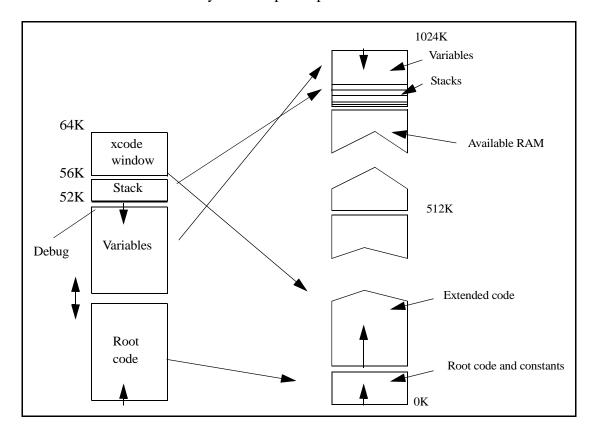
Figure 8-3. Example of Memory Mapping and Memory Usage
