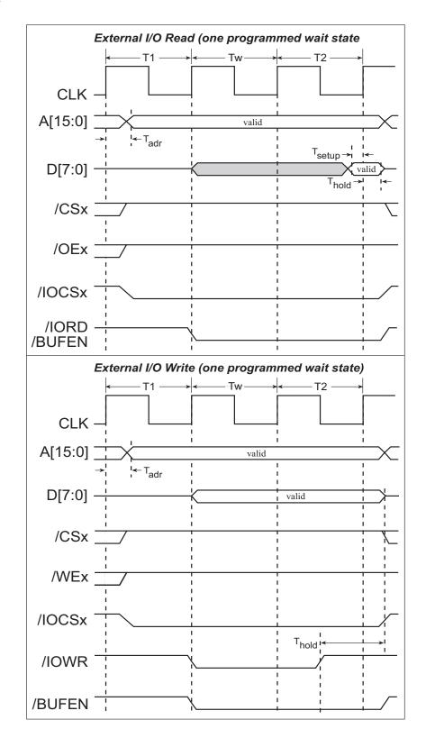
Figure 15-4. I/O Read and Write Cycles—No Extra Wait States
