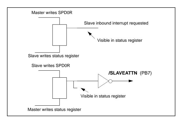
Figure 13-3. Slave Port Handshaking and Interrupts
