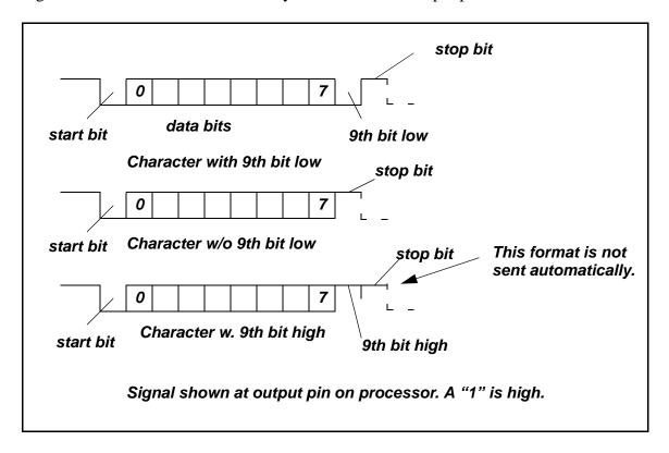
Figure 12-8. Asynchronous Serial Output Patterns
