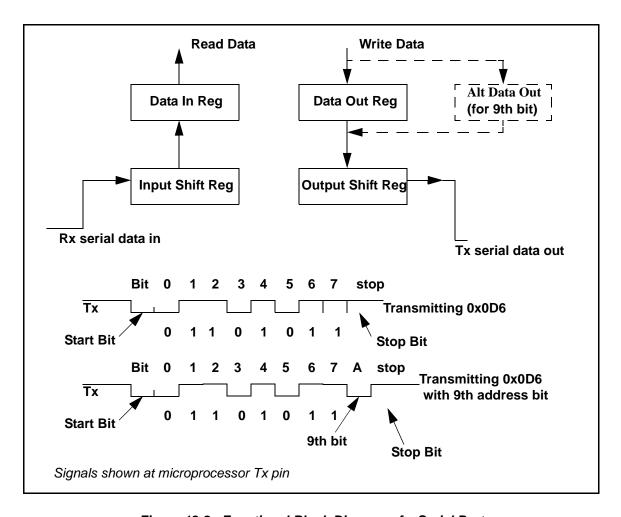
Figure 12-2. Functional Block Diagram of a Serial Port
