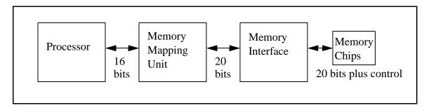
Figure 3-2. Addressing Memory Components
