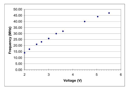
Figure 15-2. Rabbit 2000 Typical Maximum Operating Frequency versus Voltage at 25°C
