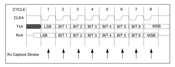
Figure 12-5. Full-Duplex Clocked Serial Timing Diagram with Internal Clock
