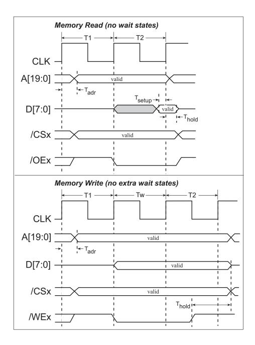
Figure 15-3. Memory Read and Write Cycles
