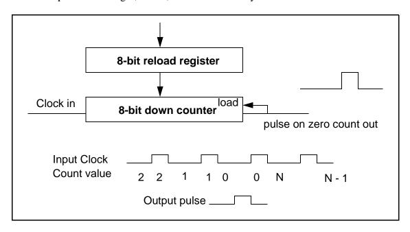
Figure 11-2. Reload Register Operation
