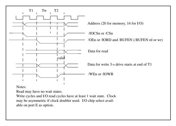
Figure 5-4. Bus Timing Read and Write
