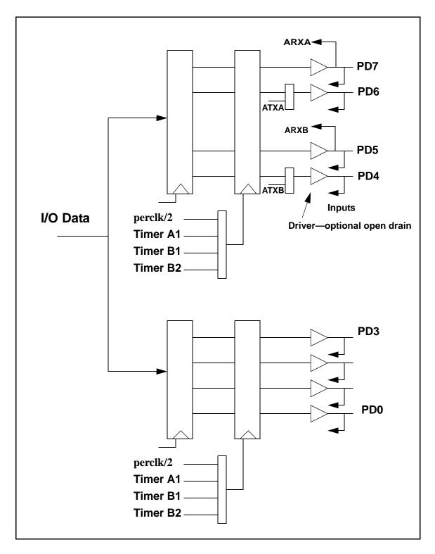
Figure 9-1. Parallel Port D Block Diagram
