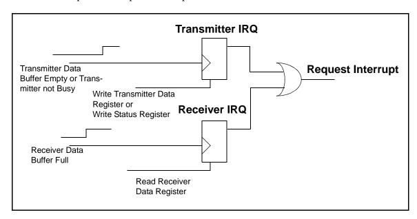
Figure 12-3. Generation of Serial Port Interrupts
