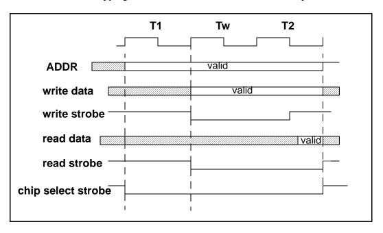
Figure 10-1. External I/O Bus Cycles
