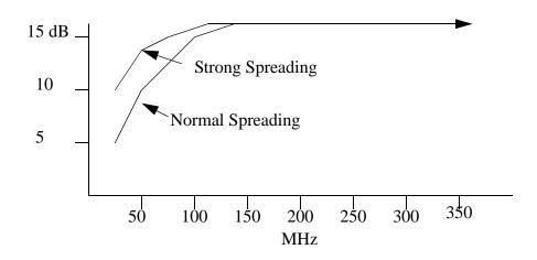
Figure B-2. Peak Spectral Amplitude Reduction from Spectrum Spreader
