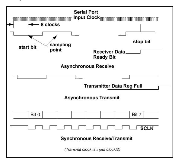
Figure 12-4. Serial Port Synchronization
