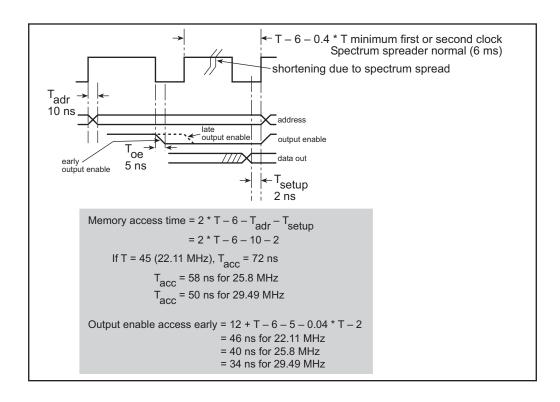
Figure B-3. Clock Spectrum Spreader Example
