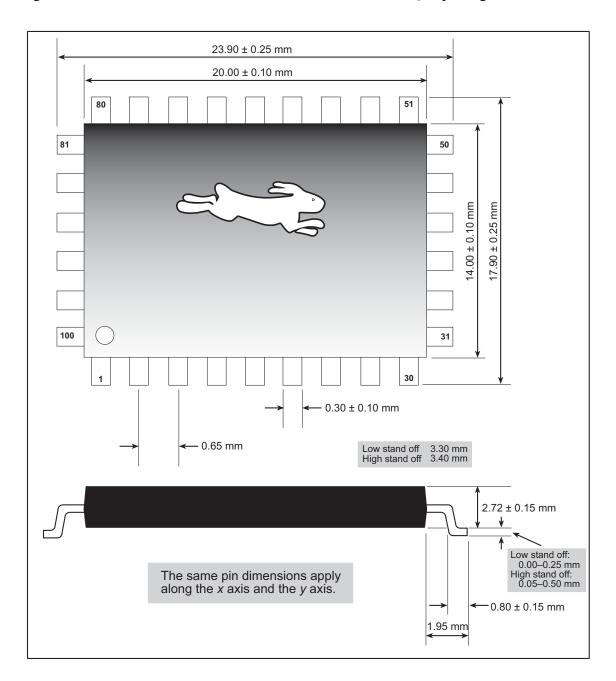
Figure 5-2. Mechanical Dimensions Rabbit PQFP Package
