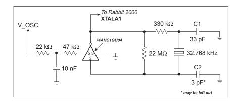
Figure B-1. Low-Power 32.768 kHz Oscillator Circuit
