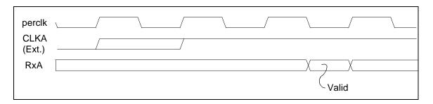
Figure 12-7. Synchronous Serial Data Receive Timing with External Clock
