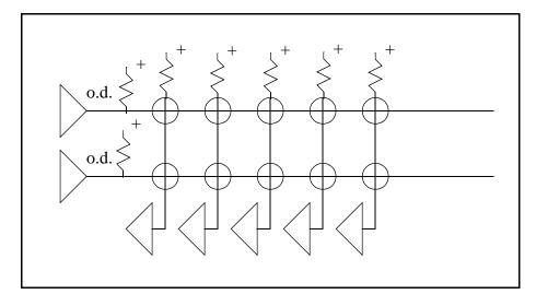
Figure 4-2. Using Open-Drain Outputs for Key Scan
