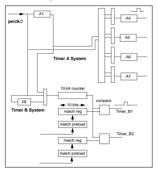
Figure 11-1. Block Diagram of Timers A and B
