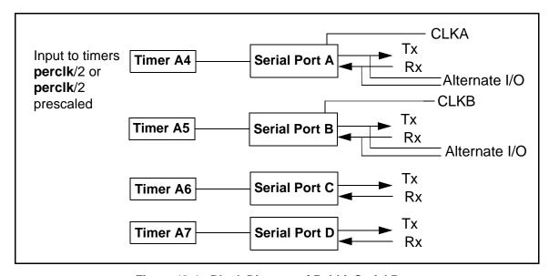
Figure 12-1. Block Diagram of Rabbit Serial Ports
