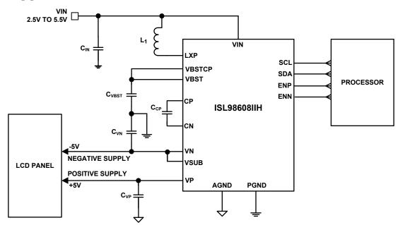
FIGURE 1. TYPICAL APPLICATION CIRCUIT: TFT-LCD SMART PHONE DISPLAY
