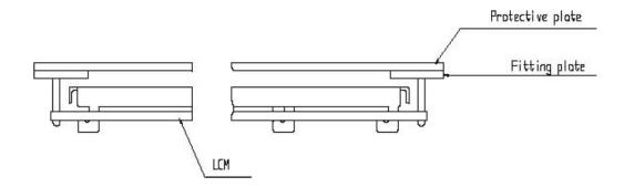
2. When assembling the LCM into other equipment, the spacer to the bit between the LCM and the fitting plate should have enough height to avoid causing stress to the module surface, refer to the individual specifications for measurements. The measurement tolerance should be  $\pm 0.1$ mm. Precaution for assemble the module with BTB connector:
