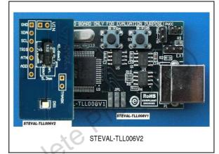
Connect the motherboard to the PC through the USB cable (AB type). Wait until the computer enumerates the control board and displays the message that new hardware has been found and is ready to use. It is then possible to run the data packet creator application by pressing the "Connect board" button.
