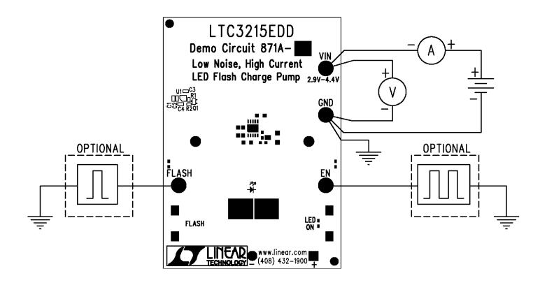
Figure 1. Proper Measurement Equipment Setup
