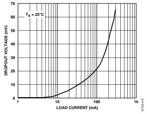
Figure 7. Dropout Voltage vs. Load Current
