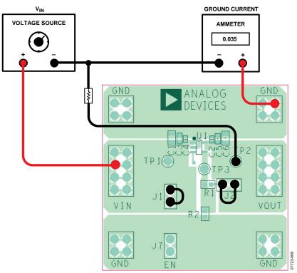
Figure 8. Configuration for Ground Current Measurements
