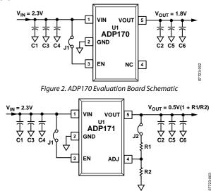
Figure 3. ADP171 Evaluation Board Schematic
