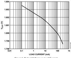
Figure 6. Output Voltage vs. Load Current
