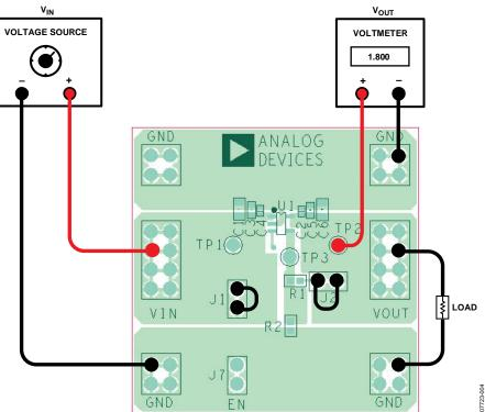
Figure 4. Configuration for Output Voltage Measurements
