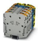
High-current terminal block, Blocked, Connection method: Power-Turn connection, Cross section: 10 mm<sup>2</sup> - 70 mm<sup>2</sup>, AWG: 8 - 2/0, Width: 80 mm, Color: gray/blue, Mounting type: NS 35/15
