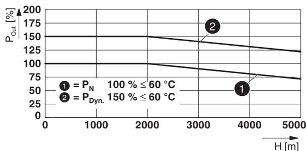
Figure 20 Output power depending on the installation height
