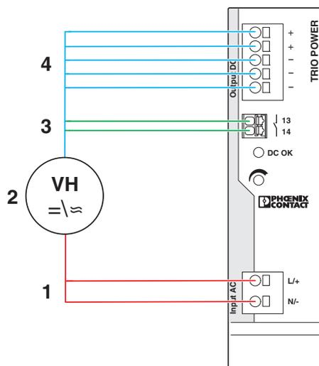
Figure 1 Potential-related wiring for the high-voltage test
