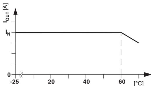
Figure 19 Temperature derating in normal mounting position
