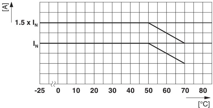
Rotated mounting position 270° Z-axis
