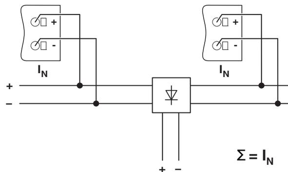
Figure 23 Schematic diagram, decoupling with diode module
