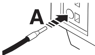
Figure 9 Insert connecting cable (push-in connection technology)
