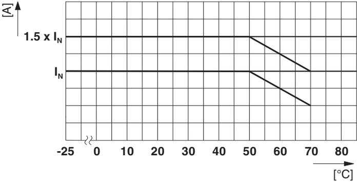
Rotated mounting position 90° Z-axis
