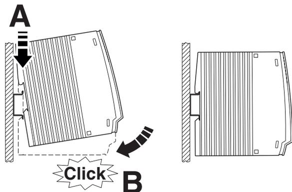
Figure 7 Assembly on standard DIN rail
