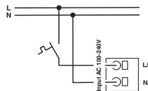
Figure 13 Schematic diagram, switching the input terminals
