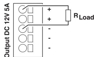
Figure 15 Schematic diagram, switching the output terminals
