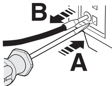
Figure 10 Release connecting cable (push-in connection technology)
