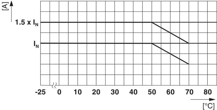
Rotated mounting position 180° X-axis
