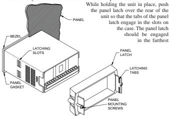
forward slot possible. To achieve a proper seal, tighten the latch screws evenly until the unit is snug in the panel (Torque to approximately 7 in-lbs [79N-cm]). Do not over-tighten the screws.
