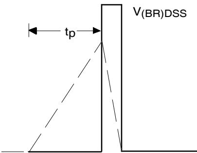
**Fig 21b.** Unclamped Inductive Waveforms
