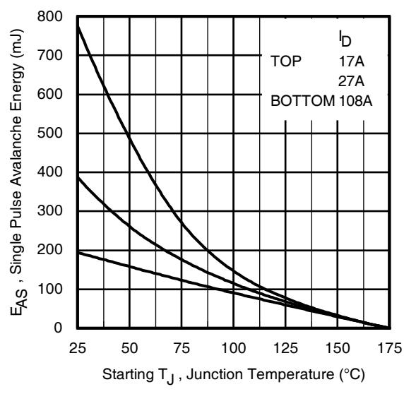
**Fig 12.** Maximum Avalanche Energy vs. Drain Current
