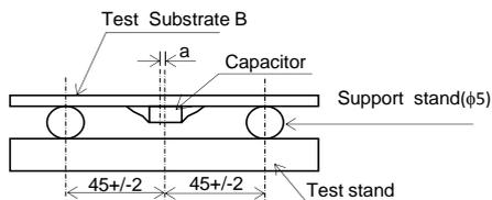
a: +/-2 gap between support stand center and test stand
