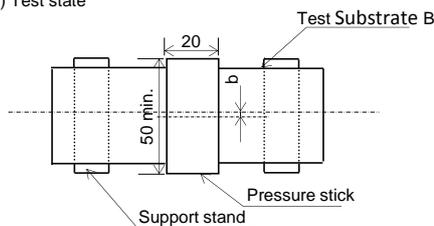
b: +/-5 gap between support stand center and test stand center
