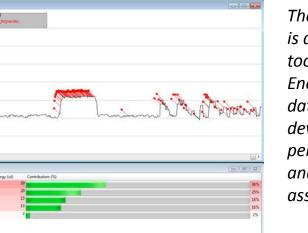
The energyAware Profiler is an energy debugging tool that use Advanced Energy Monitoring (AEM) data available from the development tools to perform real-time profiling and debugging of the associated object code.
