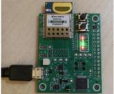
Figure 4 DWM1001 DEV board – micro USB connection
