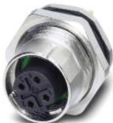
Bus system flush-type socket, Ethernet, 4-pos., M12 SPEEDCON, D-coded, rear/screw mounting with Pg9 thread, with straight solder connection, design with 12 mm long solder pins
