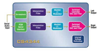
The new Cirrus Logic® family of digital-to-analog converters, the CS4344, CS4345, CS4346 and CS4348, delivers superior audio quality while providing OEMs with the industry's smallest, most cost-effective 192 kHz stereo DAC.
