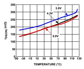
FIGURE 14. ON-RESISTANCE vs TEMPERATURE AT DIFFERENT INPUT VOLTAGES
