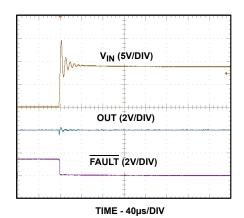
FIGURE 6. TRANSIENT WAVEFORMS WHEN INPUT STEPS FROM 0V TO 9V
