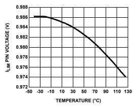
FIGURE 13. ILIM PIN VOLTAGE vs TEMPERATURE
