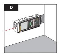
A built-in sensor automatically detects the orientation of the positioning bracket and adjusts the zero point of the instrument accordingly.
