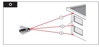
Feed Press this button **twice**; the display shows the following symbol ⊲. The laser is switched on.
