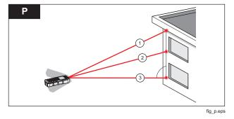
For example, determining the height between point 1 and point 2 using three target points.
