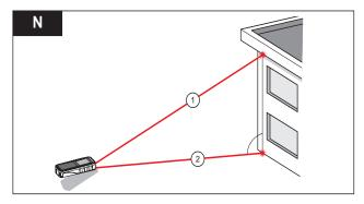
For example, for measuring building heights or widths. It is helpful to use a tripod when measuring heights that require the measurement of two or three measurements.
