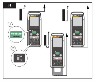
Press this button (**long** press) to set the reference to the front. Does not return to default (rear) reference.
