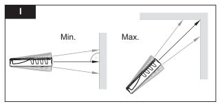
It is commonly used to measure room diagonals (maximum values) or horizontal distances (minimum values).
