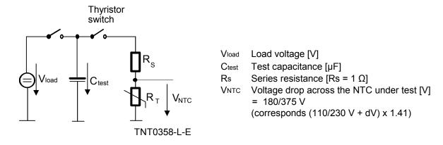
Fig. 2 Maximum switchable capacity measuring circuit
