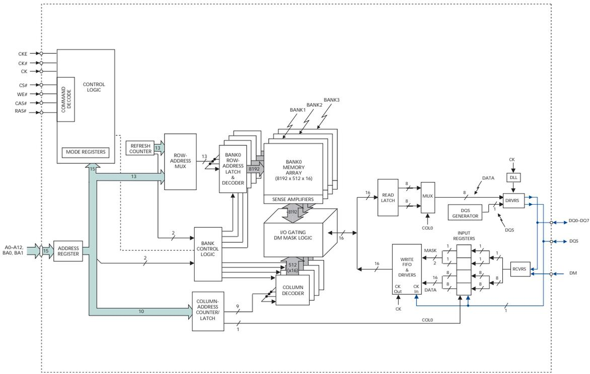
Figure 5: 16 Meg x 16 Functional Block Diagram
