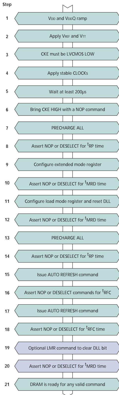
Figure 22: INITIALIZATION Timing Diagram
