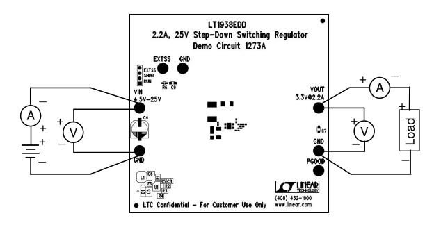
Figure 1. Proper Measurement Equipment Setup
