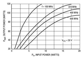
Figure 6. Output Power versus Input Power
