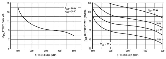
Figure 2. Power Gain versus Frequency
