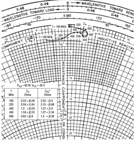
Z<sub>OL</sub>\*= Conjugate of the optimum load impedance into which the device output operates at a given output power, voltage and frequency.
