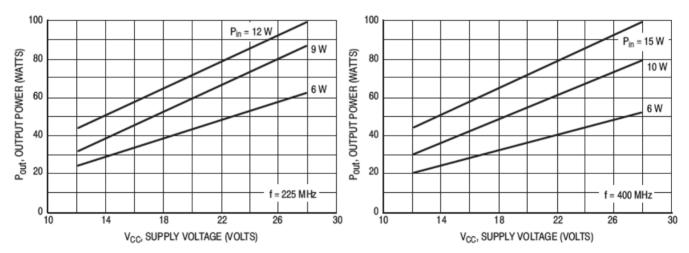
Figure 4. Output Power versus Supply Voltage
