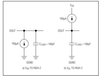
Figure 2. Load Circuit for DOUT Disable Time
