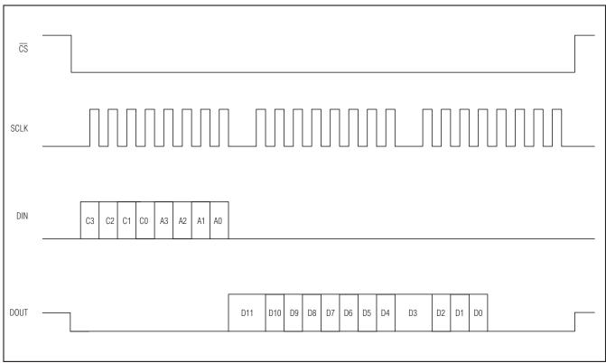
Figure 7. Serial Register Read Timing
