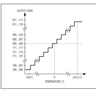
Figure 12. Temperature Transfer Function
