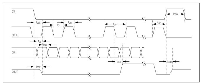
Figure 6. Detailed Serial Interface Timing Diagram
