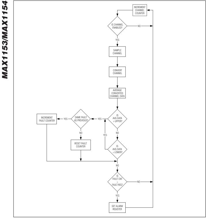
Figure 4. Alarm Flowchart
