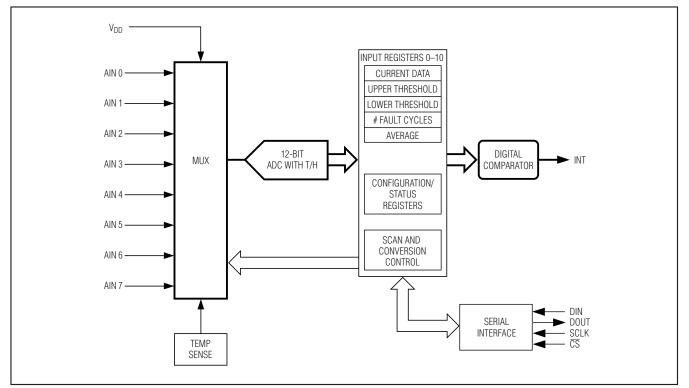
Figure 3. Simplified Alarm Block Diagram of the MAX1153/MAX1154
