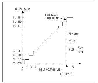
Figure 10. Unipolar Transfer Function, Full Scale (FS) = VREF
