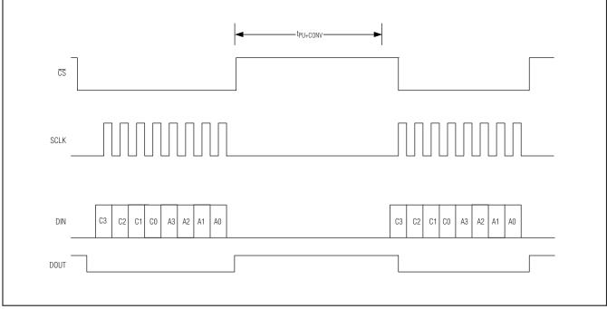
Figure 9. Manual Conversion Timing Without Reading Data
