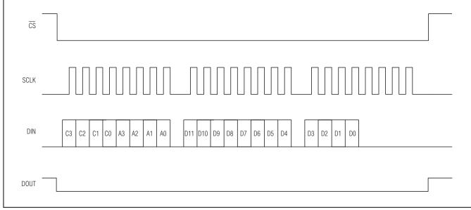
Figure 8. Serial Register Write Timing
