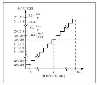
Figure 11. Bipolar Transfer Function, Full Scale (±FS) = ±VREF/2
