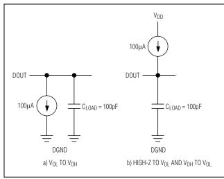
Figure 1. Load Circuits for DOUT Enable Time and SCLK to DOUT Delay Time
