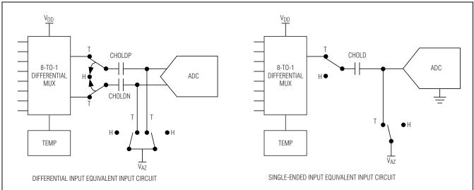
Figure 5. Single-Ended/Differential Input Equivalent Input Circuit
