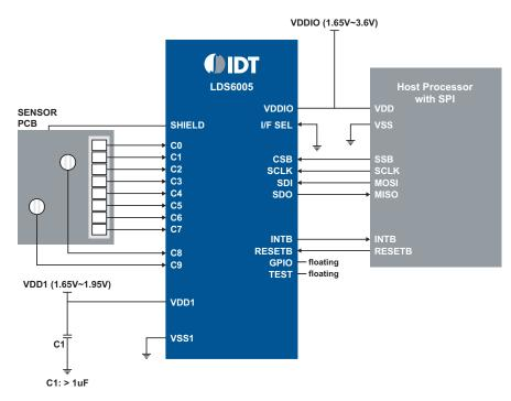
Figure 2. LDS6005 application diagram
