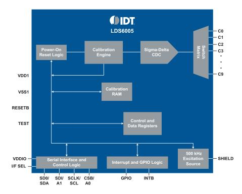
Figure 1. LDS6005 block diagram
