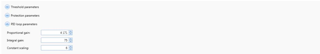
Set the PID controller factors in the torque control loop (this function is reserved for advanced users). The values given in the example below ensure correct product operation in the majority of cases.
