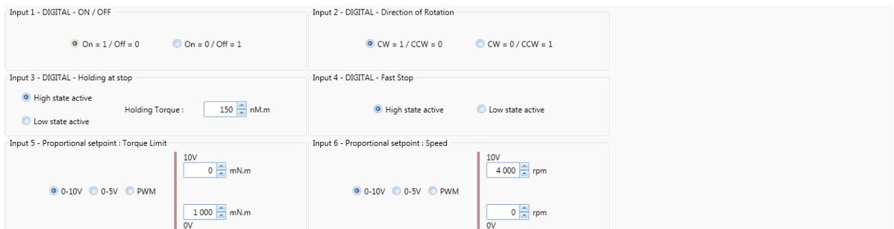
The screenshot shows the 'Inputs' tab parameters for the expert program. It is divided into six input configuration sections:
