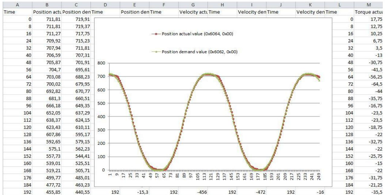
Notice that together with the channel description, you will find the internal register associated with this value. These registers are following the CANopen protocol structure since SMI21 CANopen drive is compliant with the following profiles: CiA-301, CiA-303, CiA-305, CiA-306 and CiA-402.
