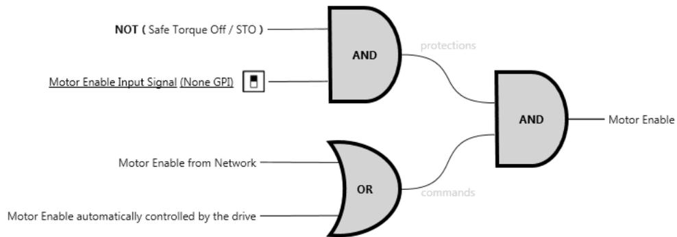
**Enable/Disable motor state is automatically controlled by the drive** parameter specifies if the motor should be automatically powered on (if possible) after power-up without the needed of user intervention.
