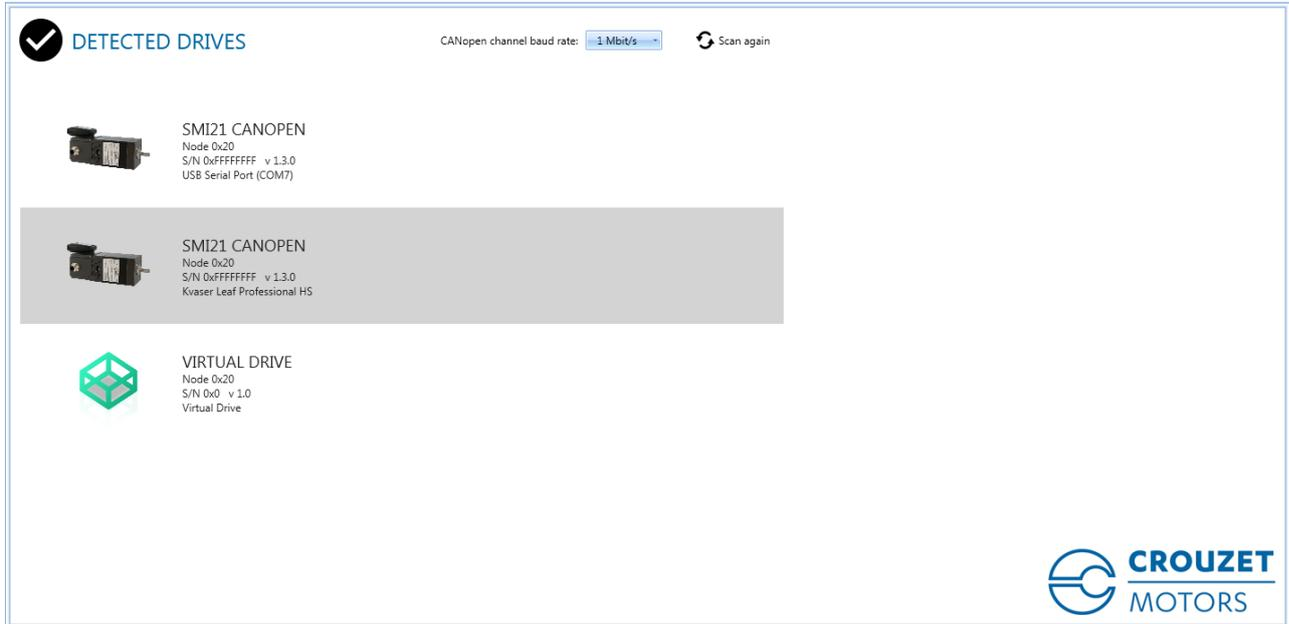
The **Drives** screen displays a list of the SMI21 CANopen drives that DCmind Soft + CANopen has found on your local network (CANopen or USB). You can select one of these drives from the list and click on the picture (grey line) to continue. This will connect you to the SMI21 CANopen drive and you will be given the option to use a wizard to setup the drive.
