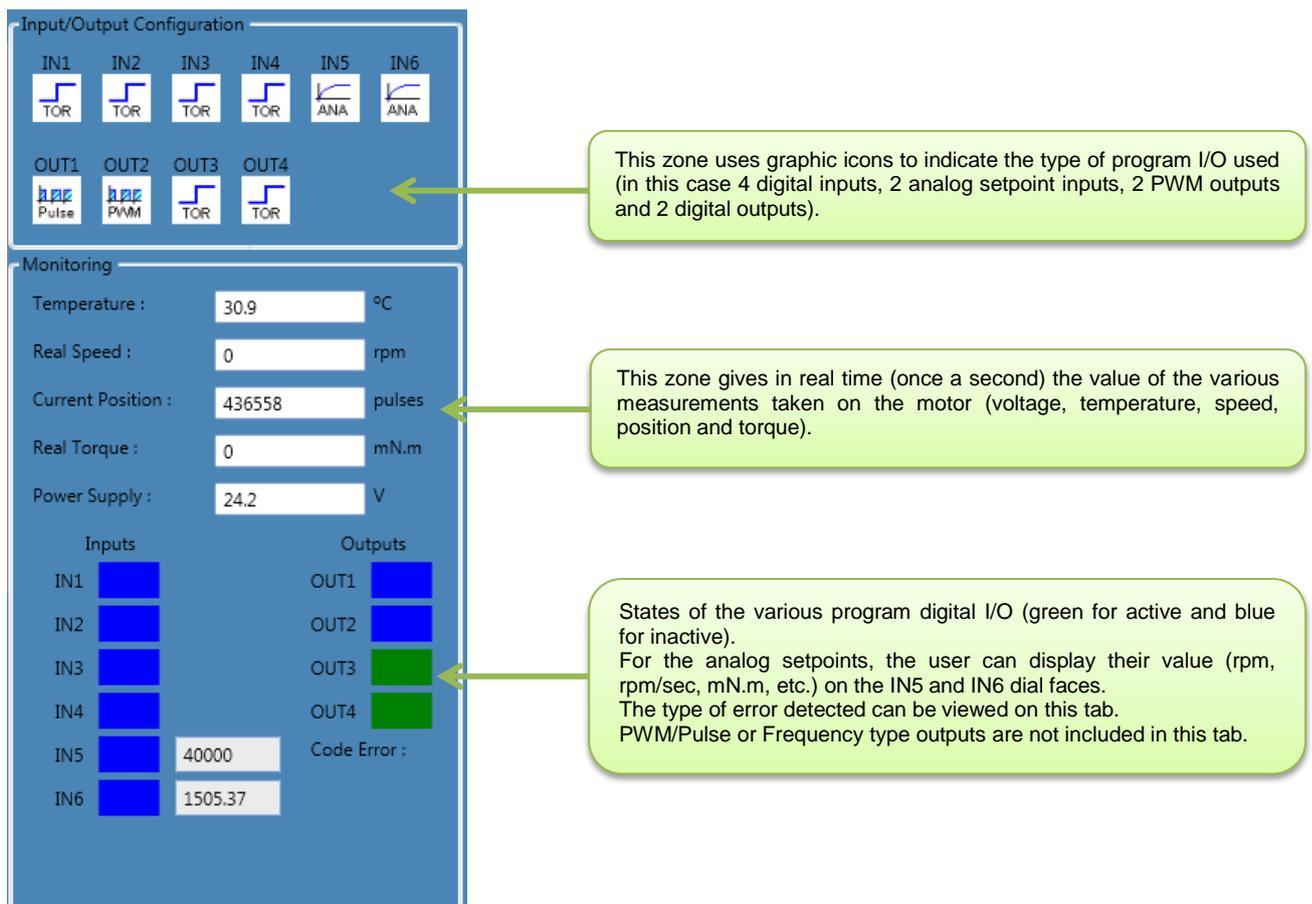
The screenshot displays the HMI monitoring window, divided into two main sections: "Input/Output Configuration" and "Monitoring".
