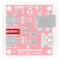
Before adding the resistor, **disconnect both jumpers** discussed in the section above. Then use this equation to select your resistor:
