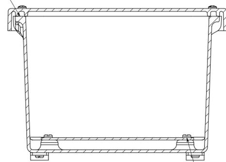
(4) EACH #10-32 BRASS INSERTS AND PLATED CARBON STEEL SCREWS
